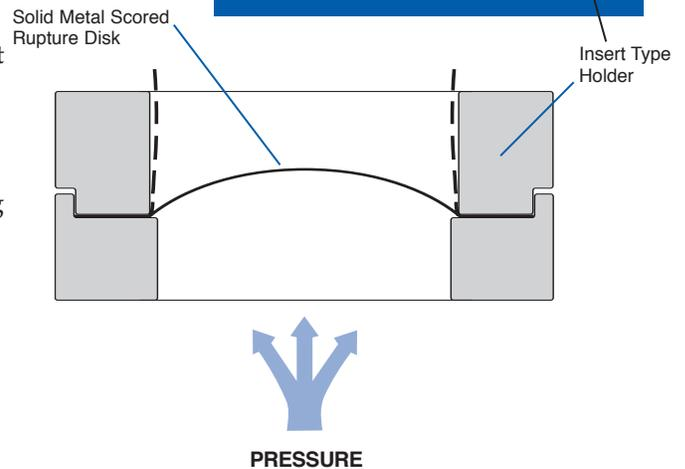
SFAZ Series Disks mount with the concave surface facing the process media. As pressure increases above the recommended operating ratio, the score lines weaken until rupture occurs. When the SFAZ Disk ruptures, the disk opens along the score lines and folds back against the holder outlet.
